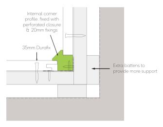
Fig. 7 - Internal corner detail
