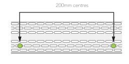
Fig. 6 - Use of perforated closure on corner profiles
