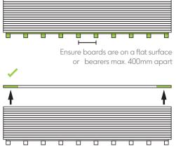
Lift boards on the edges using 2 people to lift at a time
