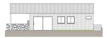
**Perforated Closures** will be needed at the top & bottom of the cladding and any windows, and the top of any doors.
