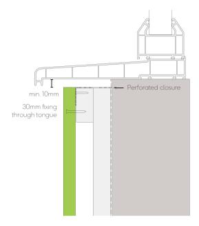
Fig. 3 - Window/door sill detail
