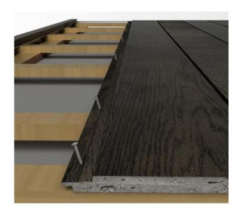
Once the first row of boards have been installed, the second row of boards can be installed beside it, with the groove covering the tongue of the previous board.
