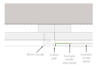
Fig. 19 - Corner profile butting upto render
