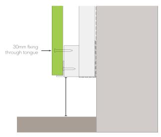
Fig. 17 - First board install
