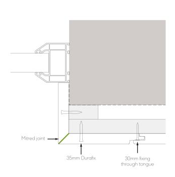
Fig. 13 - Window/door jamb with mitred joint
