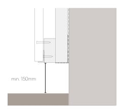
Fig. 4 - Install detail above ground level
