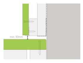
Fig. 5 - Install detail above deck
