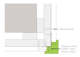
Fig. 8 - External corner detail
