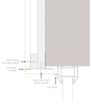
Fig. 12 - Window/door head with fascia
