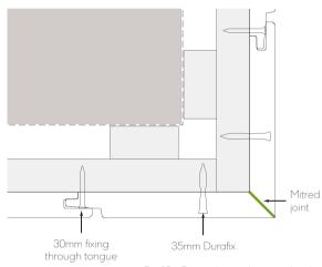
Fig. 10 - External mitred corner detail
