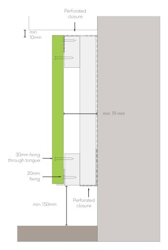
Fig.1 - Top & bottom cladding detail
