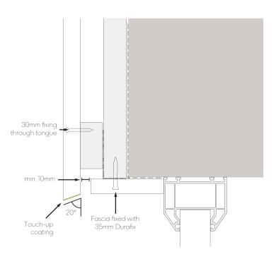
Fig. 15 - Window/door head with angled cut
