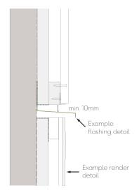
Fig. 21 - Installing cladding above render
