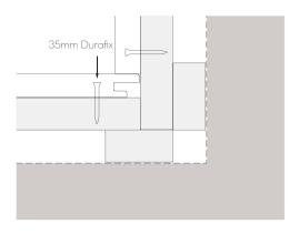
Fig. 9 - Internal butt joint corner detail
