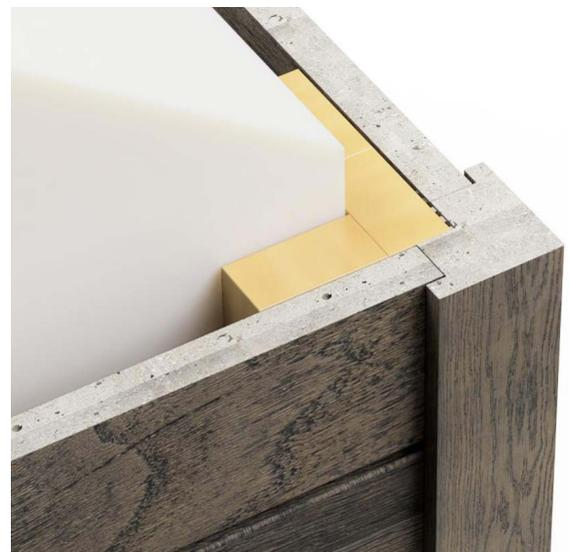
Alternatively, the boards can be butted together on an internal corner as shown in fig. 9. The boards can also be mitred to create the external corner, this would also be applicable if the corner is anything other than 90 degrees.
