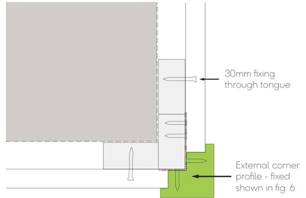
Fig. 8 - External corner detail
