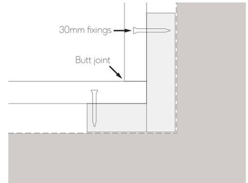
Fig. 9 - Internal butt jointed detail
