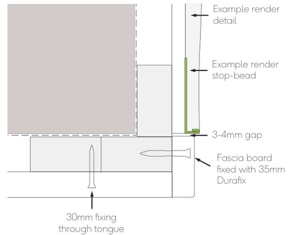
Fig. 20 - Corner profile butting up to render on external corner
