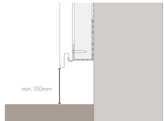
Fig. 4 - Install detail above ground level
