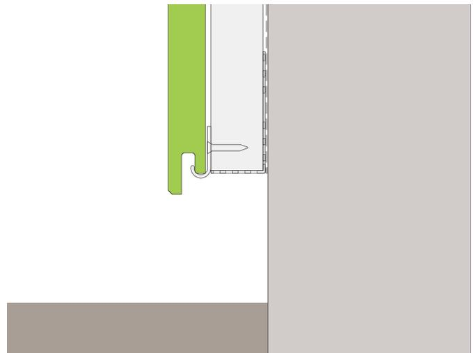
Fig. 17 - First board install
