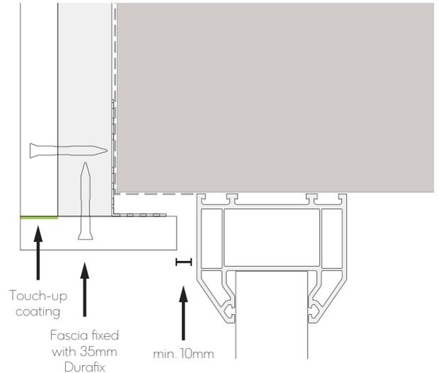
Fig. 12 - Window/door head with fascia
