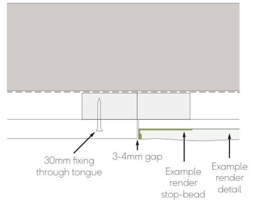
Fig. 19 - Corner profile butting up to render
