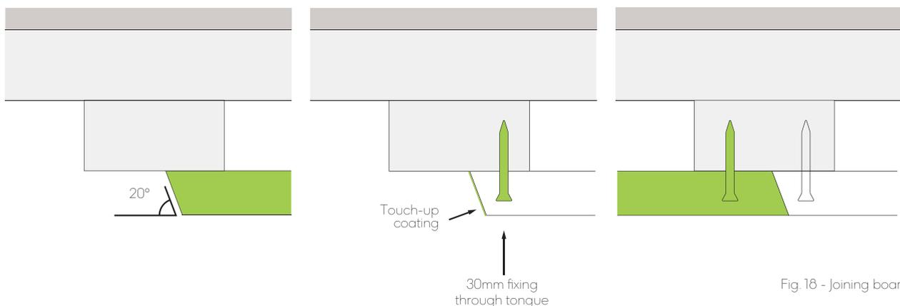
Fig. 18 - Joining boards detail
