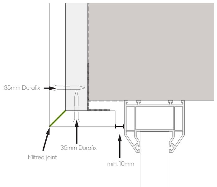
Fig. 14 - Window/door head with mitred joint
