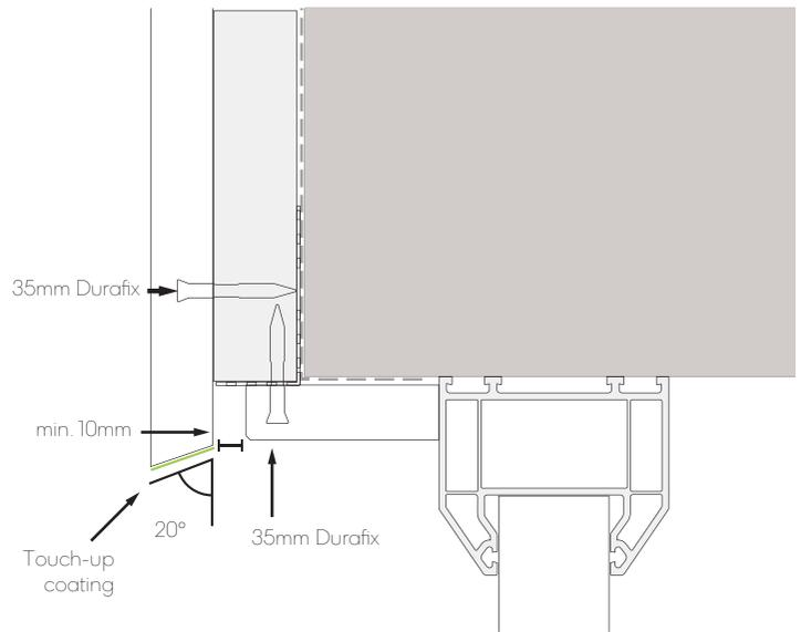
Fig. 15 - Window/door head with angled cut
